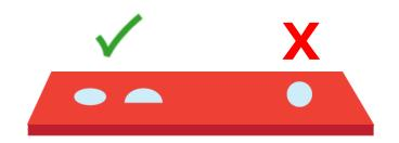
If the mold is clean, water or cleaner should wet the surface, not bead
